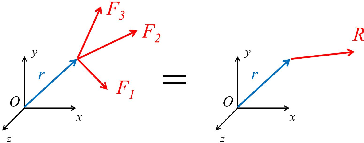
$$M_O = r \times F_1 + r \times F_2 + r \times F_3 = M_O = r \times (F_1 + F_2 + F_3) = r \times R$$
